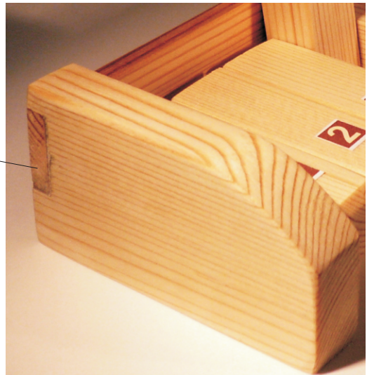
Board is butt glued
