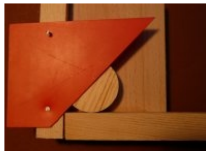
Determination of the center of the circle with a centering angle
