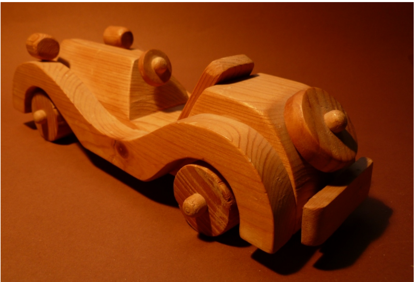
The lamps made of 20 mm spruce rods have 4 mm rods in the fenders and lamps pinned. The same procedure was followed for all wheels, the steering wheel and the spare wheel.
