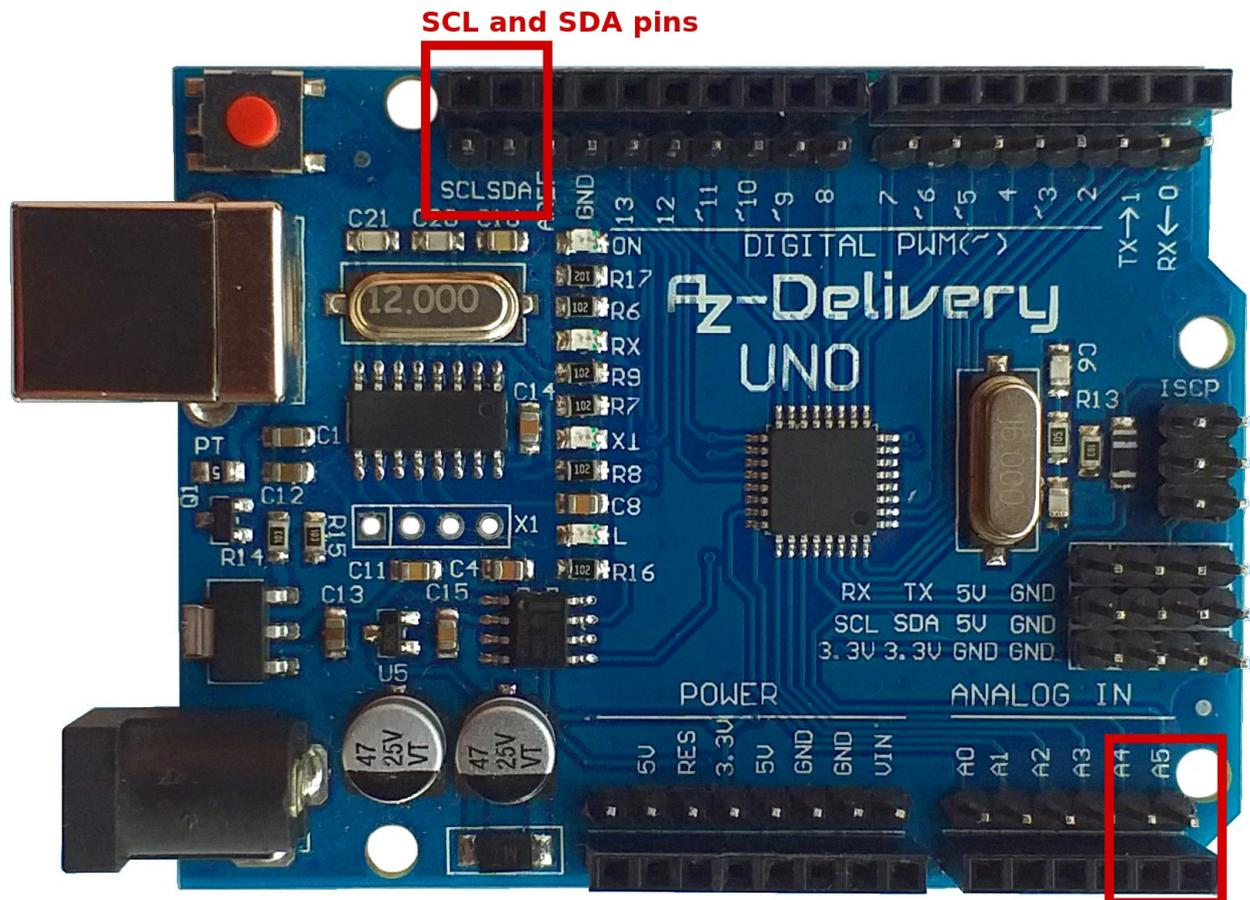
**Alternative functions of A4 and A5 are SDA and SCL connections**
